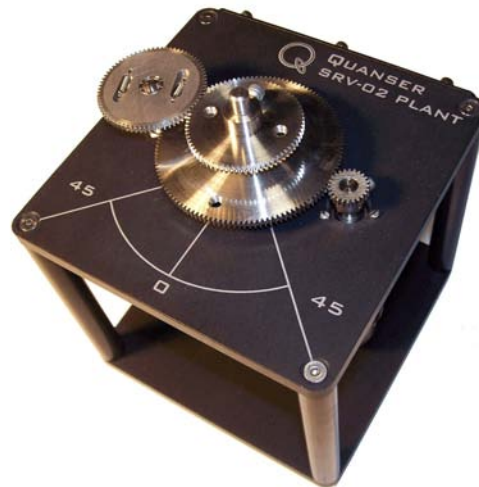
Figure 13: SRV02 in high-gear configuration.
