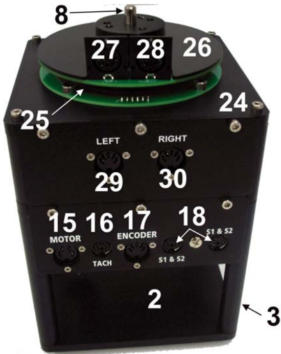
Figure 11: Components on the SRV02-ETS.
