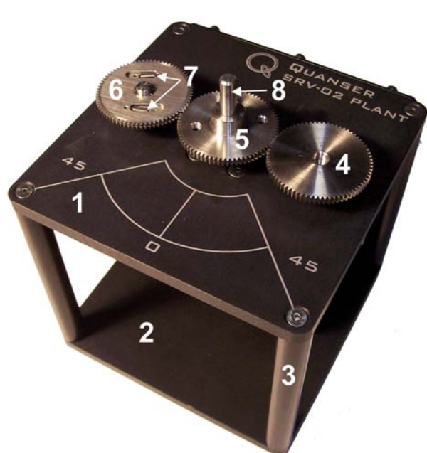
Figure 2: Top view of components on the SRV02 in low-gear configuration.
