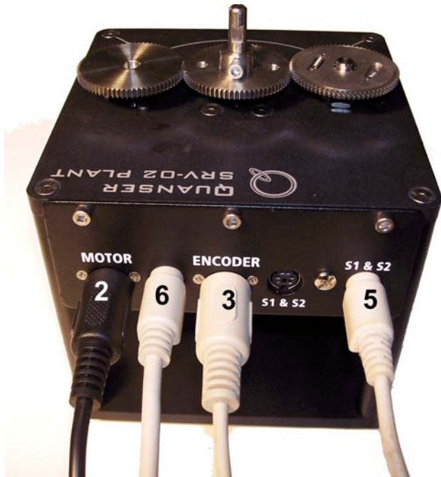
Figure 23: Connections on the Quanser SRV02 device.
