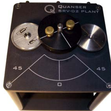
Figure 15: SRV02 with disk load attached.
