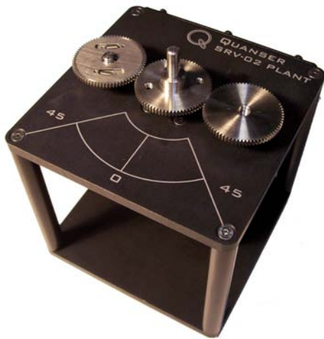
Figure 12: SRV02 in low-gear configuration.
