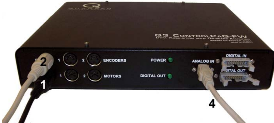
Figure 24: Connection on Q3.
