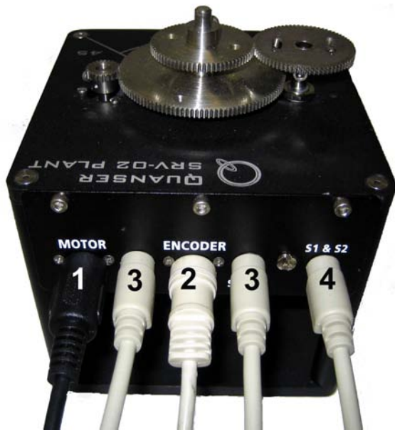
Figure 25: Connections on SRV02 from Q3.
