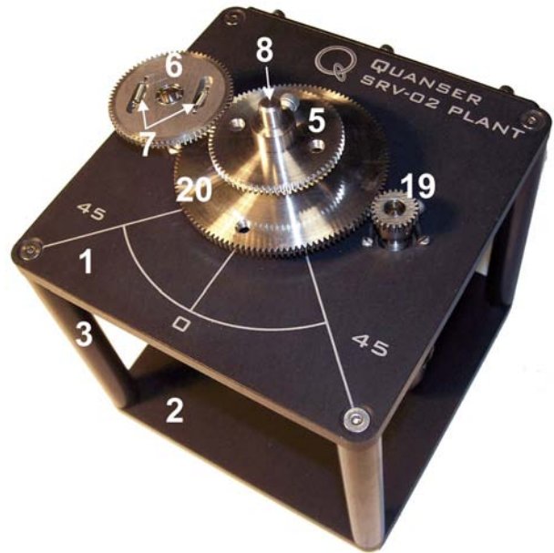
Figure 5: Top view of the components on the SRV02 in high-gear configuration.
