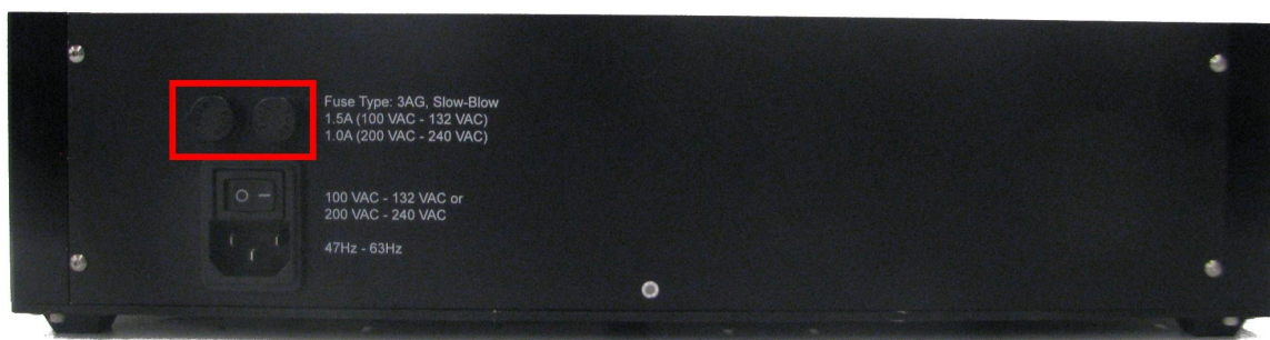
Figure 8: Backside of VoltPAQ-X2 has 2 fuses.
