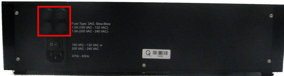
Figure 9: Backside of VoltPAQ-X4 has 4 fuses.
